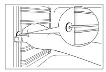
2. Pull the rear shelf support rail away from the side wall and remove it.
